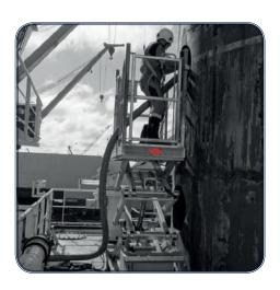
For platforms used outside we recommend a galvanized solution as it does not rust.
